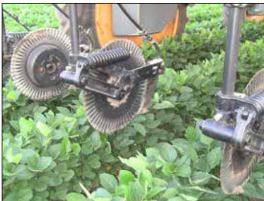
Figure 4. Coulters/Knife injection in 30" rows.
