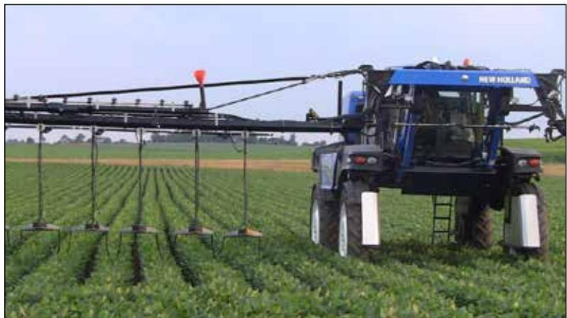
Figure 2. New Holland equipped with YDrop™.
